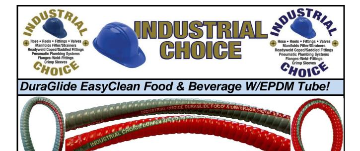
DuraGlide with EPDM Tube is designed to convey Food & Beverage items, with acidity like juice, wine, spirits, vinegars and will handle harsh cleaning agents. When deciding which tube is best consider: Cleaning/Sanitizing Solutions and acidic products can deteriorate Chlorobutyl & Nitrile rubbers making them flake off, gumming up your filters and damaging product. An EPDM FDA rubber offers better resistance to these acidy products and cleaning agents.
